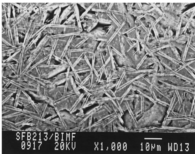
Fig. 1 SEM photo of MACOR sample annealed for 2 h at 930 °C
