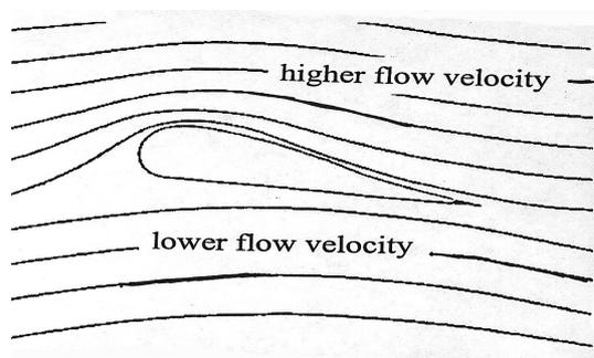
**Figure 1:** Airflow around an airfoil.
