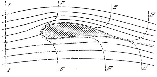
**Figure 7:** Position of originally adjacent air particles during the flow around a profile at consecutive times I, II, III, IV.
