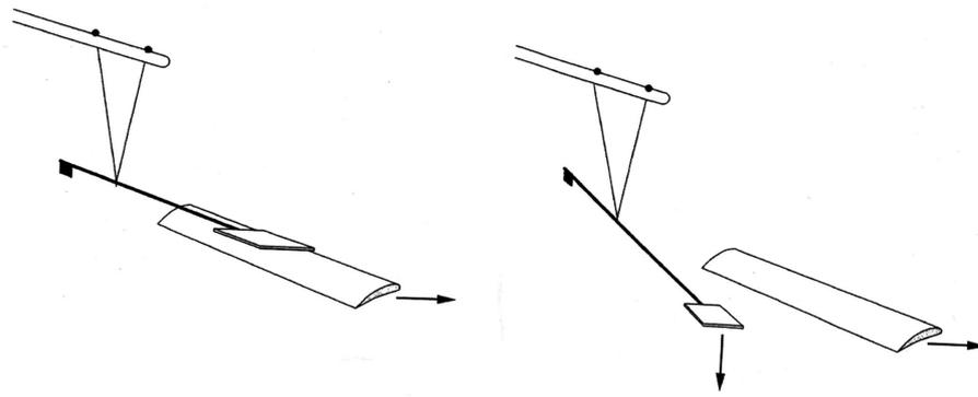
**Figure 3:** Indicator of air movement. Left: Position of cardboard before and while passing of the airfoil. Right: Vertical movement of the cardboard indicating vertical movement of the air induced by the airfoil. Wood lath: Cross section about 5 mm x 5 mm, length about 1 m. Airfoil about 15 cm x 60 cm.
