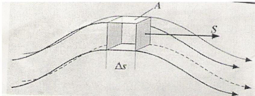
**Figure 4:** Tangential acceleration of a volume within curves stream lines.
