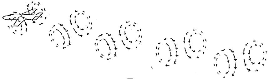
**Figure 8:** System of vortices behind an airfoil
