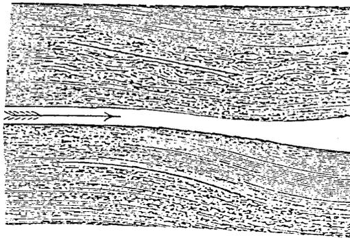
**Figure 6:** Deflection of airflow by an even plane and a curved plane.
